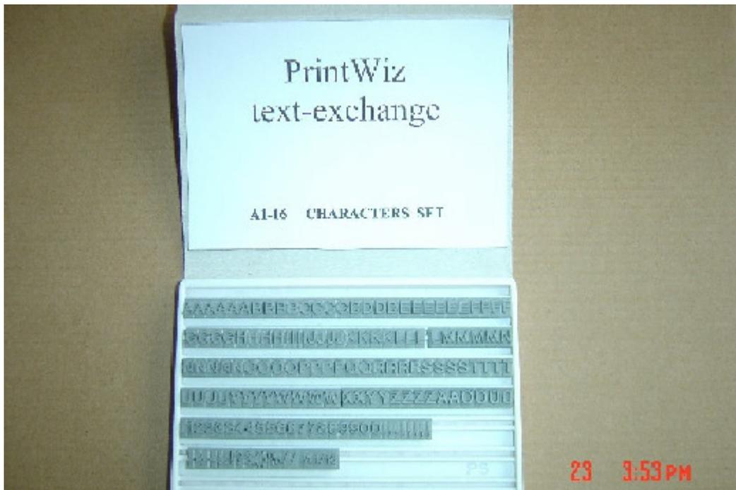
In addition to permanent information placed on the printing wheel, our system allows to insert and replace at will, additional (limited) information, on our specially designed printing wheel. The character set is available as an optional extra, together with **PFT.** (**P**rintwheel **F**or **T**ext).
